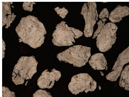
Fig. 1 Maraging powder particles after 20 h milling
